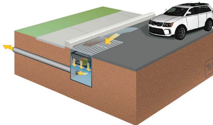
Figure E-13 Typical Distributed Source Control Structural BMP Schematic (arrows indicate water pathways)
